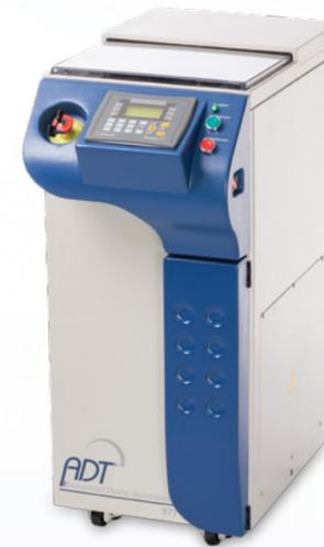
Designed for after-dicing workpiece cleaning and drying. Equipped with a spinning chuck table and a rotating washing/drying arm. The arm can be configured with an atomizing cleaning nozzle or a high pressure nozzle to cope with a wide range of cleanliness requirements.
